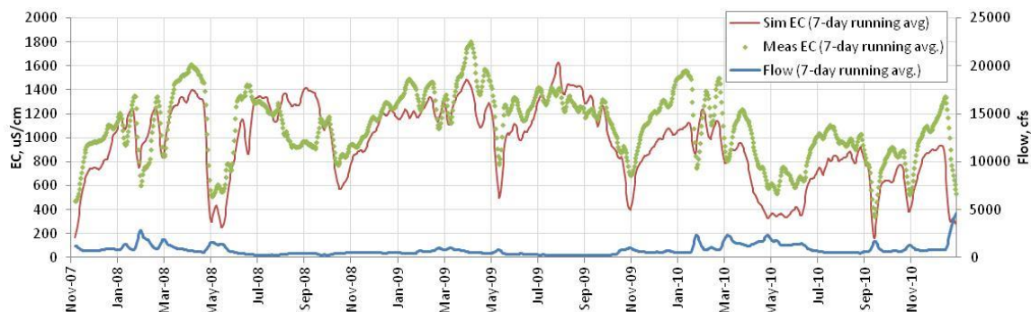
Figure 3. Comparison of simulated and measured EC in San Joaquin River at Crow's Landing after calibration (2008-2010). Simulated flow profile at that location is presented on the secondary axis.
